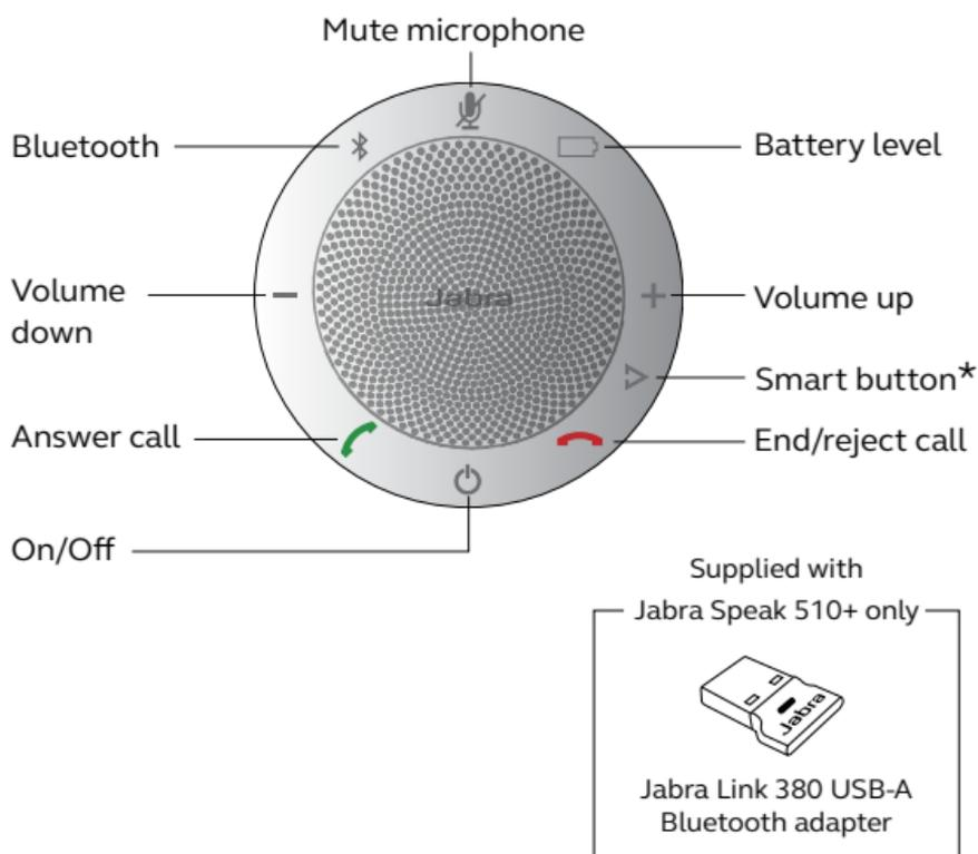
\*Newer Speak 510 variants (with the Smart button) have a Ver. ID beginning with D, or later. Older Speak 510 variants (without the Smart button) have a Ver. ID beginning with A, B, or C.
